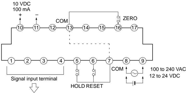
**Note:** Terminals 7 to 13 are connected internally.
