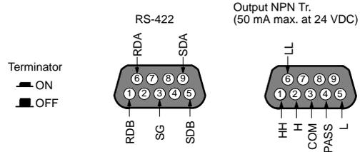
**K31-FLK4: RS-232C + Transistor (NPN Open Collector)**
