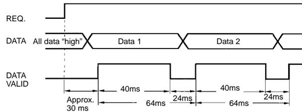
The K3NV outputs each measurement at an interval of 64 ms when a REQ signal is ON continuously.
