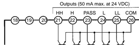
**K31-T2: Transistor (PNP Open Collector)**
