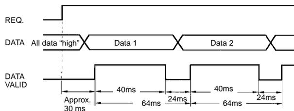
The K3NX outputs each measurement at an interval of 64 ms when a REQ signal is ON continuously.
