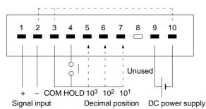
Note: 1. Terminals 2 and 3 and 10 are not internally insulated. Connect a relay with high contact reliability and insulation (with a minimum load current of 0.3 mA) or a photocoupler with high insulation (with a residual voltage of 1 V max. and a current leakage of 0.1 mA max.) to these terminals for external control. The use of an independent power supply is recommended for the Digital Panel Meter.
