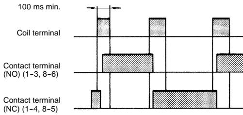
**Note:** When a pulse for application to the coil is used, such a pulse should have a width of 100 ms or more. If a pulse is applied with a width less than the operate time, the cam may fail to rotate fully.
