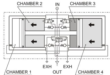
When the down stream pressure decreases, the pressure booster starts again its alternating cycle till a new balance condition is restored. The pressure booster can be furnished complete with pressure regulator installed on the inlet port for getting an accurate outlet pressure value. A wall mounting plate is also available.
