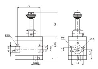
Flow adjusting needle for needle for progressive filling
