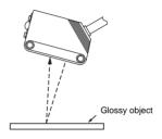
If there is a mirror-like object below the Sensor, the Sensor may not operate stably. Therefore, incline the Sensor or separate the Sensor from the mirror-like object as shown below.
