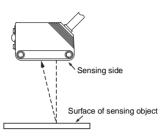
If the sensing object has a glossy surface, however, incline the Sensor by  $5^\circ$  to  $10^\circ$  as shown in the illustration, provided that the Sensor is not influenced by background objects.
