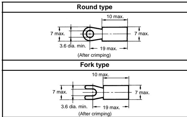
**Note:** Use terminals with insulation tube (recommended crimp terminal: 1.25 to 3.5).
