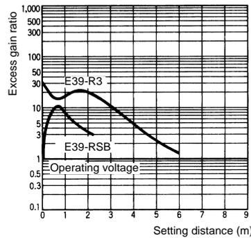
**Excess Gain Ratio vs. Setting Distance (Typical)**
