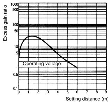
**Excess Gain Ratio vs. Setting Distance (Typical)**
