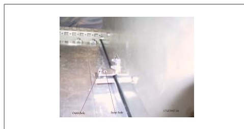
Illustration 4.30: Move mounting screws from the outer hole to the inner hole
