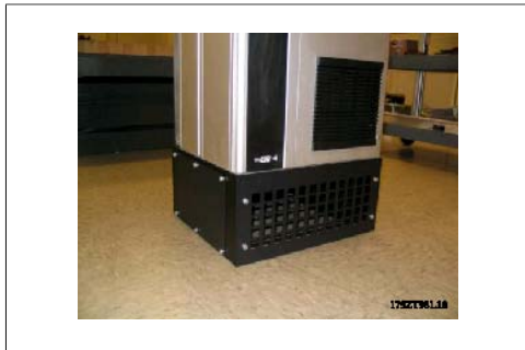
Illustration 5.8: Frame D2 with pedestal installed
