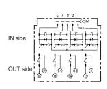
Note: Do not reverse the coil polarity.
