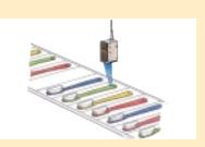
Sorts toothbrushes by the color of their handles. Stable detection can be obtained without being influenced by changes in brightness of sensing objects.
