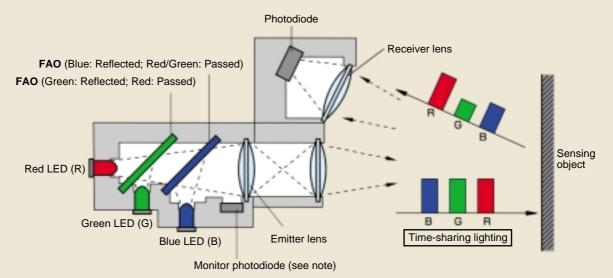
Note: The monitor photodiode compensates LED output deviation that may be caused by a temperature change.
