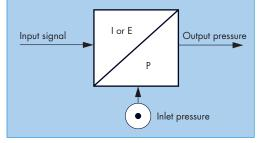
The key to the MAC PPCs are two MAC 34, 45, 400, 47, 92 or 93 Series valves that are used to control the output pressure. The valves are operated by the PPCs closed loop electronic control circuit. Feedback is obtained from one or two transducers. The balanced poppet, fast response, and high flow of these two MAC Valves provide outstanding performance characteristics for the PPC.
