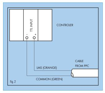
There also is a negative logic version (LMS) available. When the correct pressure is achieved, this option outputs a logic 0. When the PPC is working (fill or exhaust valve is in operation) the output is a logic 1. In either case, the LMS circuit is a sinking type of output. Thus, the PPC supplies the ground to the reading device.
